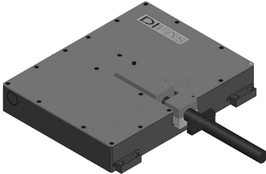
Fig. 6 3D drawing of prototype T-Bar module with high power fiber adapter.
