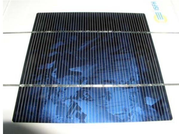
Fig. 6: With In-Laminate Laser Soldering (ILLS) manufactured solar cell module
