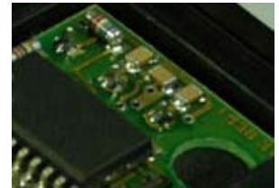
Via soldering in hard to reach places
