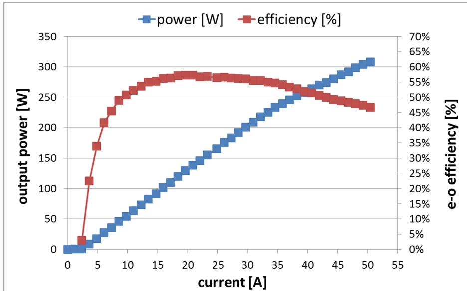
Fig. 8: P-I-E diagram for the light-weight module.
