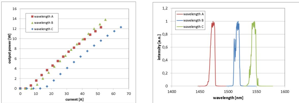
Fig.3.: individual P-I-curves and spectra for the three bars combined in a single fiber output of  $400\mu\text{m}$ , NA0.22
