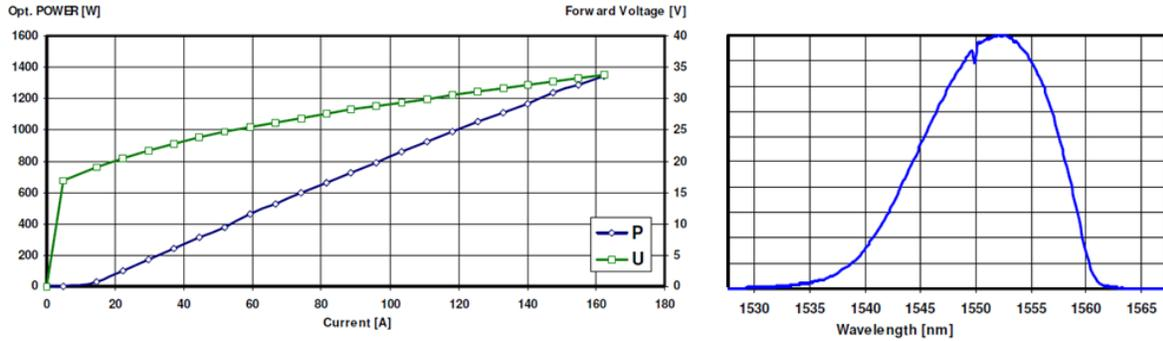
Fig. 5: results are shown for a QCW, conduction cooled 20-bar stack at 1550nm, operating at 70W peak power per bar (1%dc, 60Hz)
