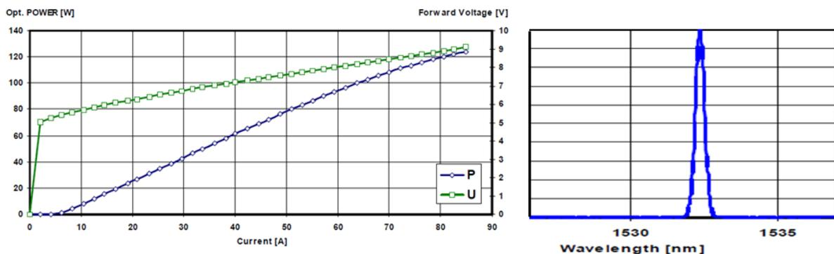
Fig. 4.: spectrally line narrowed, fiber-coupled module ( $400\mu\text{m}$ , NA0.22), based on six conduction cooled bars at 1532nm,  $\square\square < 0.5\text{nm}$  FWHM.
