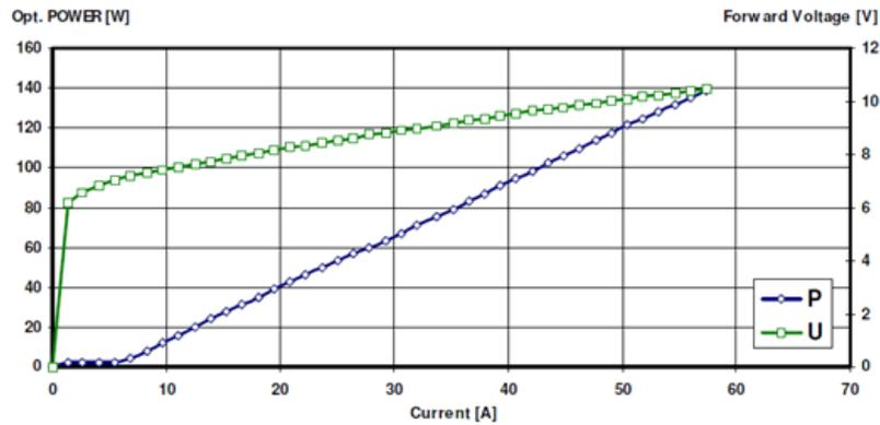
Fig. 6: PUI-curve of a 10-bar, 150W micro-channel cooled CW stack, operating at 1920nm, at 20°C, WPE of >22%.
